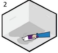
Dry and absorbent substrate should be pre-wet with water or treated with **Diamond Acrylic Primer.**
