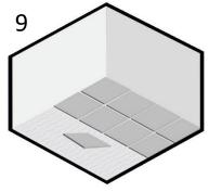
2 days after application the surface is ready for tiling, rendering or application of screed. **Diamond Seal T80** is not recommended as the final top coat.
