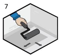
When first layer is touch-dry the second layer of **Diamond Seal T80** is applied. It is important that the second layer is applied perpendicular to the first layer.
