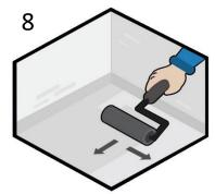
In areas subject to increased water pressure such as swimming pools and water tanks it is recommended to apply a third layer of **Diamond Seal T80**.
