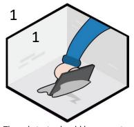
The substrate should be concrete or cement based floor screed. Holes, cracks and weak parts should be repaired with cement based mortar before water proofing.
