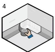
Mesh is fitted into the first layer of **Dimond Seal T80**, 50mm on both sides of the corner or joint.
