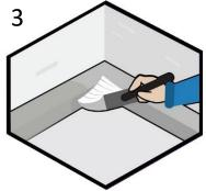
All corners and joints are brushed with one layer of Diamond Seal **T80** at minimum 50 mm on each side of the corner.
